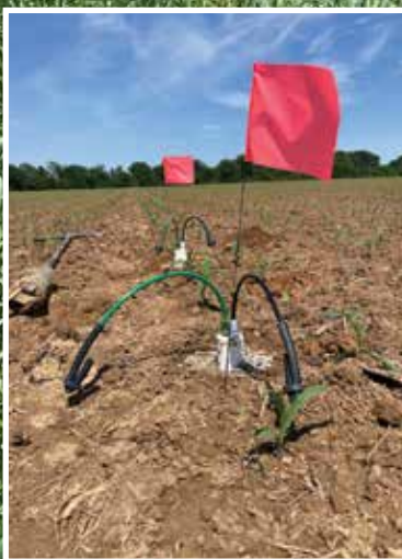
Above: Lysimeters were installed in each test plot to collect water samples.
