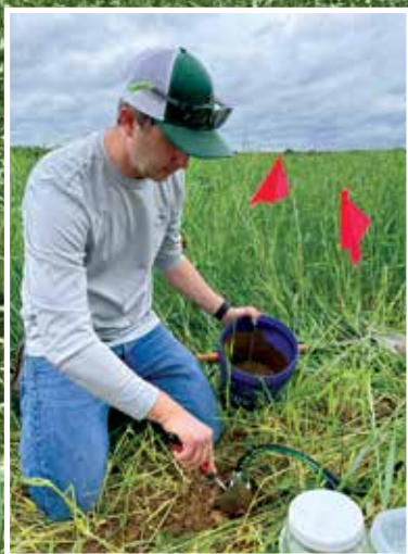
Director of Agriculture & Restoration Tim Rosen installs a lysimeter in a local farm field treated with biostimulants.
