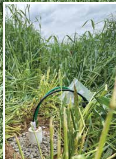
Above: Lysimeters were installed in each test plot to collect water samples.
