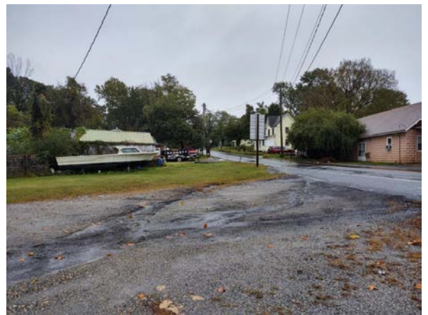
Figure 33. This bioretention would be located on a property owned by the Maryland State Highway Authority. At present, the area is just gravel. Stormwater from Old Wye Mills Rd. and Route 404 sheet flows across the gravel. The bioretention would capture and infiltrate the stormwater. It is suggested that a stormwater sewer be added to this area to help convey any excess stormwater not handled by the bioretention.
