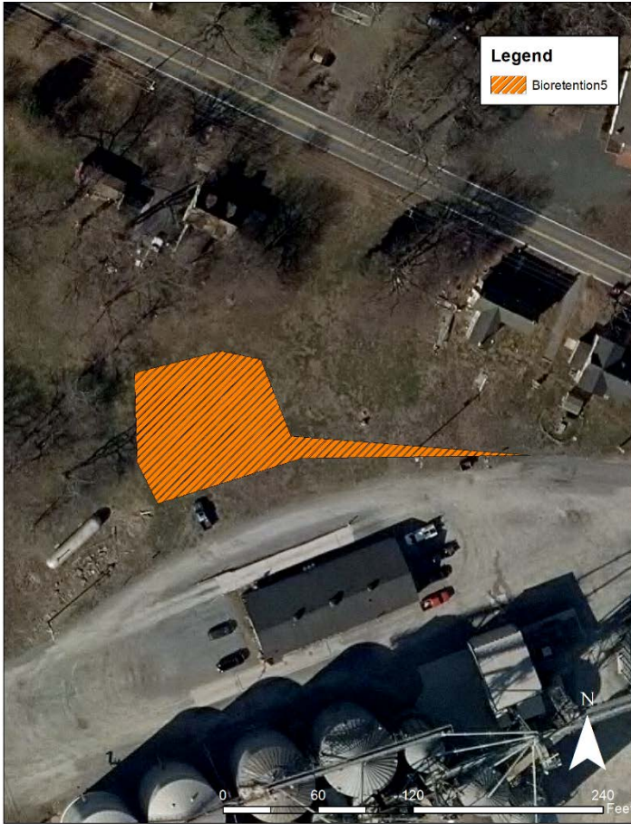
Figure 30. This bioretention would collect water from the parking area at Nagel Grain. There are no stormwater practices in this area at present, and water goes down a small hill toward Route 404.
