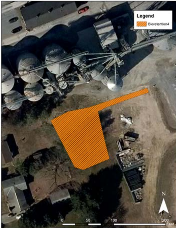
Figure 31. This area receives water from the Nagel Grain facility, and at present there are no stormwater practices. The water sits in small a grassy area and when it builds up high enough it will flow down along the property line to Old Wye Mills Rd. The proposed bioretention will help better infiltrate the water and also reduce the stormwater volume flowing off the property onto the road.
