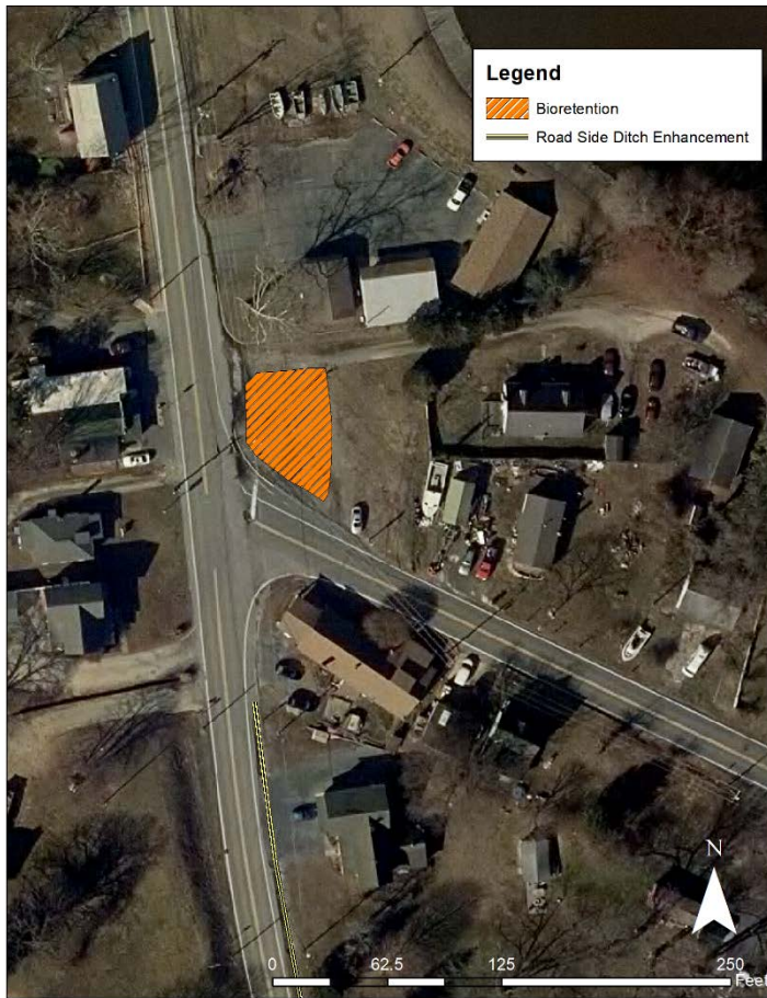
Figure 33. This bioretention would be located on a property owned by the Maryland State Highway Authority. At present, the area is just gravel. Stormwater from Old Wye Mills Rd. and Route 404 sheet flows across the gravel. The bioretention would capture and infiltrate the stormwater. It is suggested that a stormwater sewer be added to this area to help convey any excess stormwater not handled by the bioretention.
