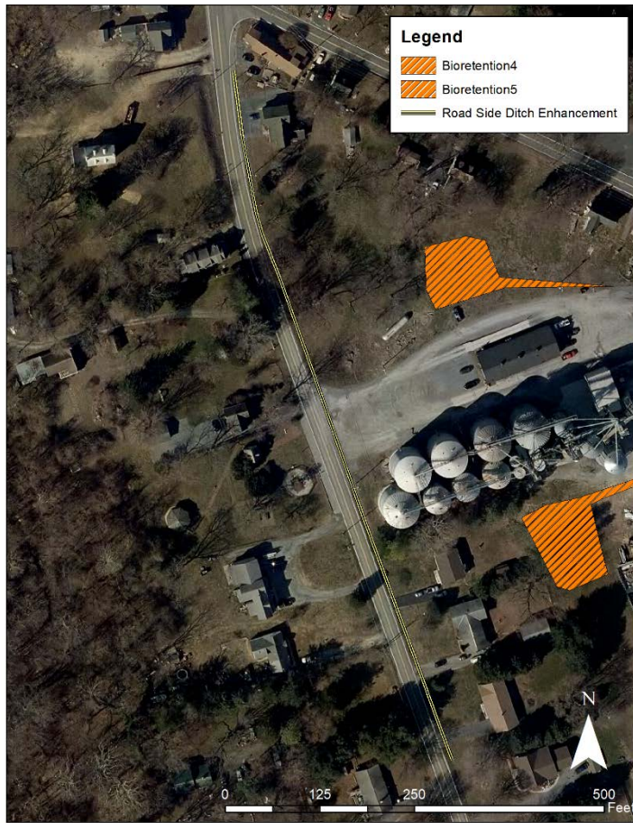
Figure 32. The current roadside ditch is shallow and in need of repair. There are multiple culverts for each driveway that in some instances are blocked. The ditch abruptly ends at the intersection of Old Wye Mills Rd. and Route 404, causing sheet flow across the roads during storm events. This ditch enhancement would reshape the ditch so that it can convey water in a less problematic manner, help better infiltrate water to reduce stormwater volume, and add a stormwater drain at the end so water does not sheet flow across the road.
