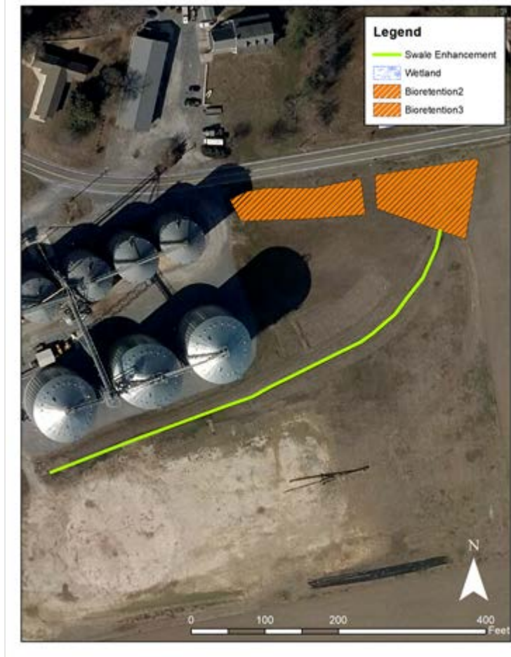
Figure 29. The grassed swale with check dams is already existing. This project would simply enhance the swale to act more like a bioswale by enhancing portions of the swale with more permeable media.
