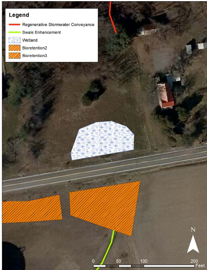
Figure 26. This potential wetland area is already enrolled in a continuous Conservation Reserve Program (CRP) easement. At present, the area is grassed. The proposed wetland/stormwater storage area is located where stormwater enters the field from the road. This project would fit within CRP guidelines and also provide necessary stormwater retention to reduce/meter water volume entering the RSC.
