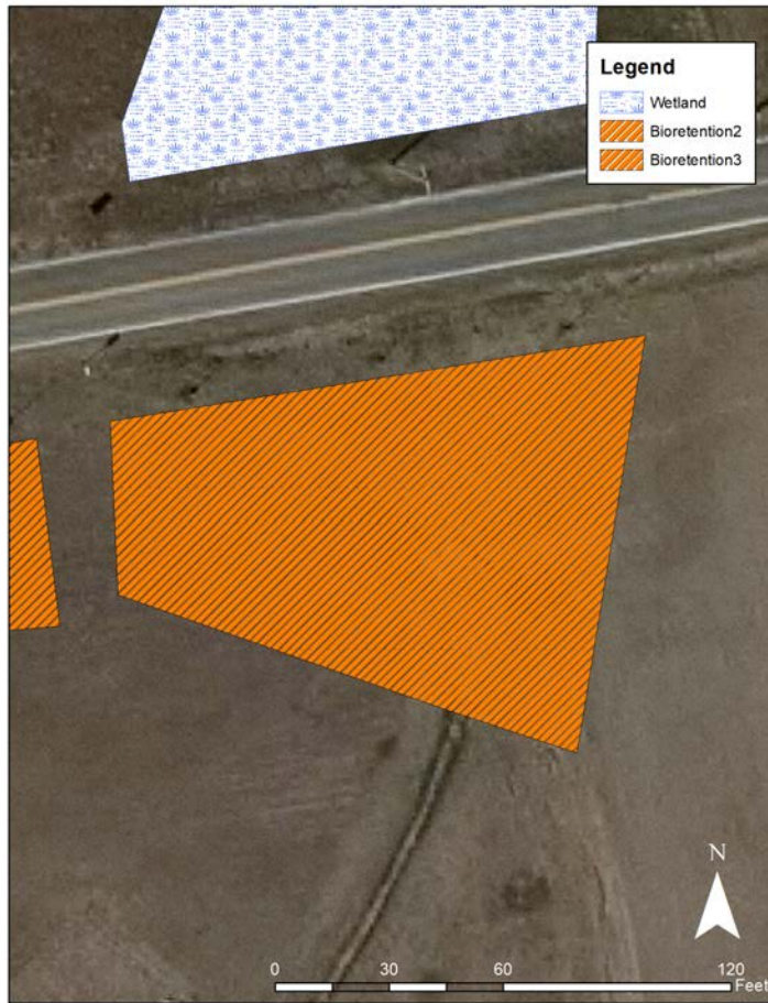
Figure 27. This bioretention would receive water from an existing grassed swale that collects water from the Nagel Grain facility. The bioretention could potentially be designed to intercept water from the adjacent farm field. The outlet of the bioretention would need to go under Route 404 in a pipe with an outlet into the proposed wetland area. The bioretention to the west of this site could be tied into this bioretention if elevations permit.
